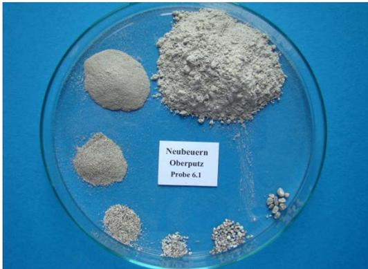
Fig. 3: Final plaster coat sample 6.1
