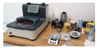
Fig. 2: Planetary Micro Mill PULVERISETTE 7 premium line
