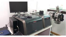
Fig. 3: Particle Sizing ANALYSETTE 22 and a Cross Beater Mill PULVERISETTE 16
